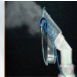
Competitor masks express aerosol as shown upward to the eyes Note: tested at 8 LPM
